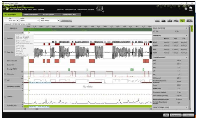
6. WM100TD and WM090TD devices only: To view the current device settings at the time of an event, move the mouse into the green bar in the area above the event.
