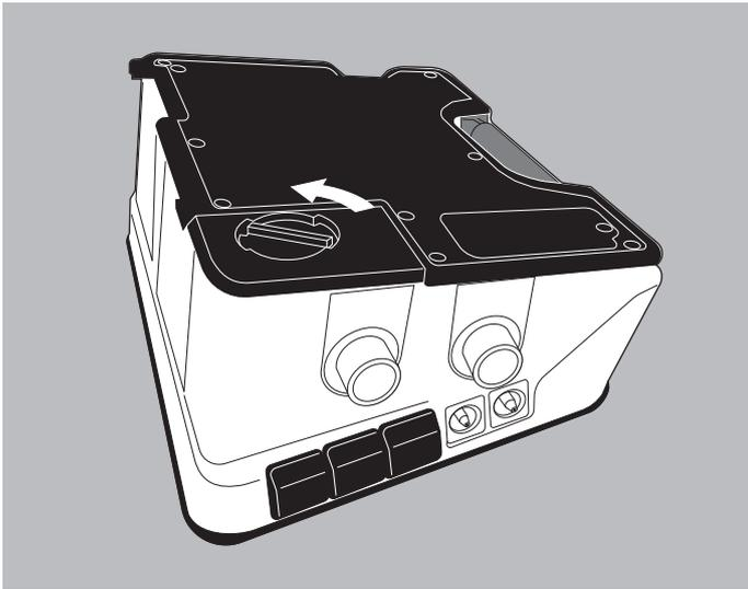
1. To open the exhalation module compartment on the rear of the device, turn the latch counterclockwise to the symbol.
