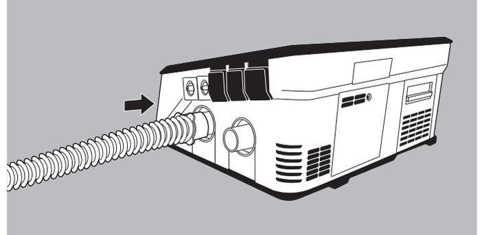
2. Push the inspiration tube onto the device outlet port.
