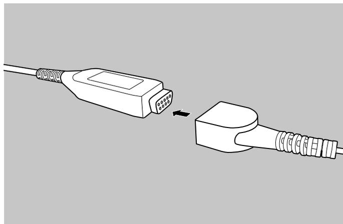
1. Connect the SpO<sub>2</sub>/Xpod<sup>®</sup> cable to the SpO<sub>2</sub> sensor.
