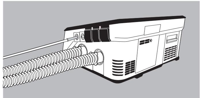
1. Push the inspiration tube onto the device outlet port.
