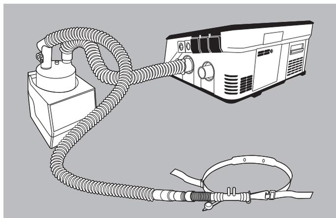
1. Push inspiration tube (short tube) onto the device outlet.
