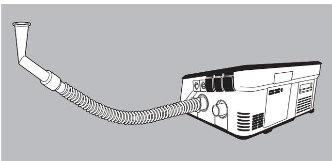
1. Push the free end of the leakage circuit onto the device outlet. It is likewise possible to use a single circuit with valve or a double circuit.
