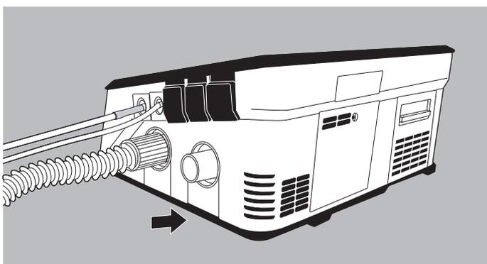
1. Push the inspiration tube onto the device outlet port.
