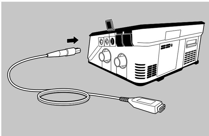
2. Connect the SpO<sub>2</sub>/Xpod® cable to the device.
