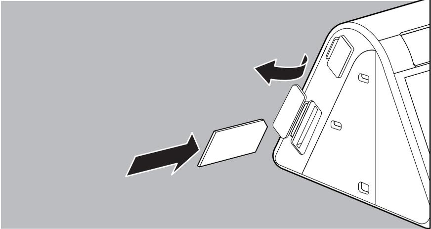
2. Push the SD card into the SD card slot until you hear it engage.
