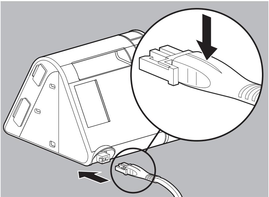
2. Plug the free plug on the power supply unit connecting cable into the power supply connection on the therapy device. Make sure the plug is aligned correctly.
