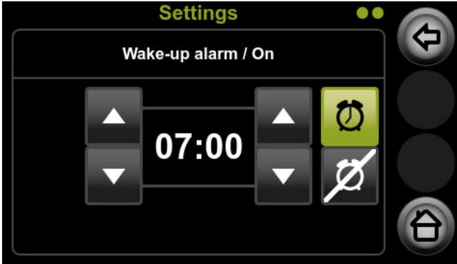
5. To set the wake-up time, use the left arrow keys to select the hours and the right arrow keys to select the minutes.
