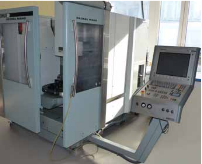
Milling machine for the production of aluminum forms
